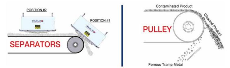
Davis Industrial understands how serious it is protecting your product and equipment from foreign objects. Permanent separators help separate tramp ferrous metals from conveyed material. They are typically suspended above the belt, which allows them to effectively and efficiently pull metal up and away from the product flow before discharging it safely away from the conveyor.
