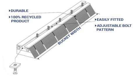
Material: steel belted bus and truck tires or solid rubber
